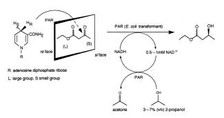
Fig. 9. Stereochemistry of PAR [17] and a schematic representation of the PAR reduction process.
