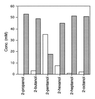
Fig. 3. Effect of secondary alcohols on (R)-CCE production. Each secondary alcohol was added to the reaction mixture at 5% (v/v) instead of 2-propanol as described in Fig. 2. The amount after 24 h of (R)-CCE produced from 1% (53 mm) m-CCP was drawn as a grey bar, and m-CCP remaining as a white bar. Complete conversion was observed for 2-propanol. The data are the average of three measurements.
