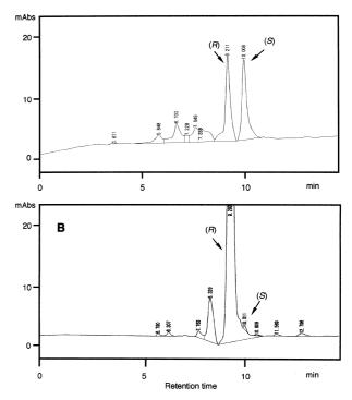
Fig. 6. HPLC analysis of CEE enantiomers. (A) Racemic CEE standard. (B) Enzymatically produced (R)-CEE (19). Each sample was loaded on a column of Chiralcel OB-H ( $4.6 \times 250$  mm), which was attached to a Shimadzu LC-10AT HPLC system, and analyzed under the conditions as described in Materials and methods.
