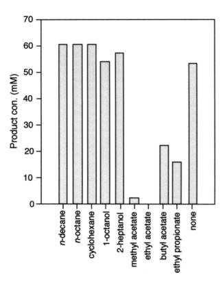
Fig. 7. Effect of organic solvent on the production of (R)-ECHB with a two-phase system. The whole reaction mixture consisted of 50% (v/v) organic solvent, 1% (61 mm) ECOB and 5% (v/v) 2-propanol, 25  $\mu$ mol KPB, 0.5  $\mu$ mol NAD<sup>+</sup>, and 60 mg of E. coli cells in a total volume of 1 mL. The bar indicates the (R)-ECHB produced from 1% ECOB after 24 h. Complete conversion was observed for n-decane, n-octane and cyclohexane.
